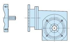
Worm Gearbox with Input Flange Motor
