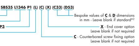
Part Number Beam Length L = 1346 mm Precision grade: options are P1, P2 & P3 L - Lightweight beam option for SB S Leave blank if not required
