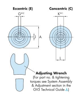
The Blind Hole Fixing type (BH) allows mounting into a solid machine base where through mounting is not possible, or where adjustment from the front is preferred. They are available in Concentric type (C), which are fixed, and Eccentric type (E), which are adjustable.
